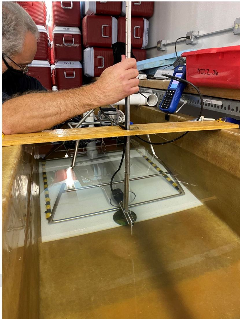
Figure 2-3 Swim Speed Chamber with Flow Meter Deployed
